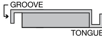
Begin laying your floor in the left corner of the longest wall. Start by placing the first panel with the groove side to the wall. Use spacers along each wall to maintain an expansion space of 8–12 mm (3/8"–1/2") between the wall and the flooring. **Diagram 1.**
